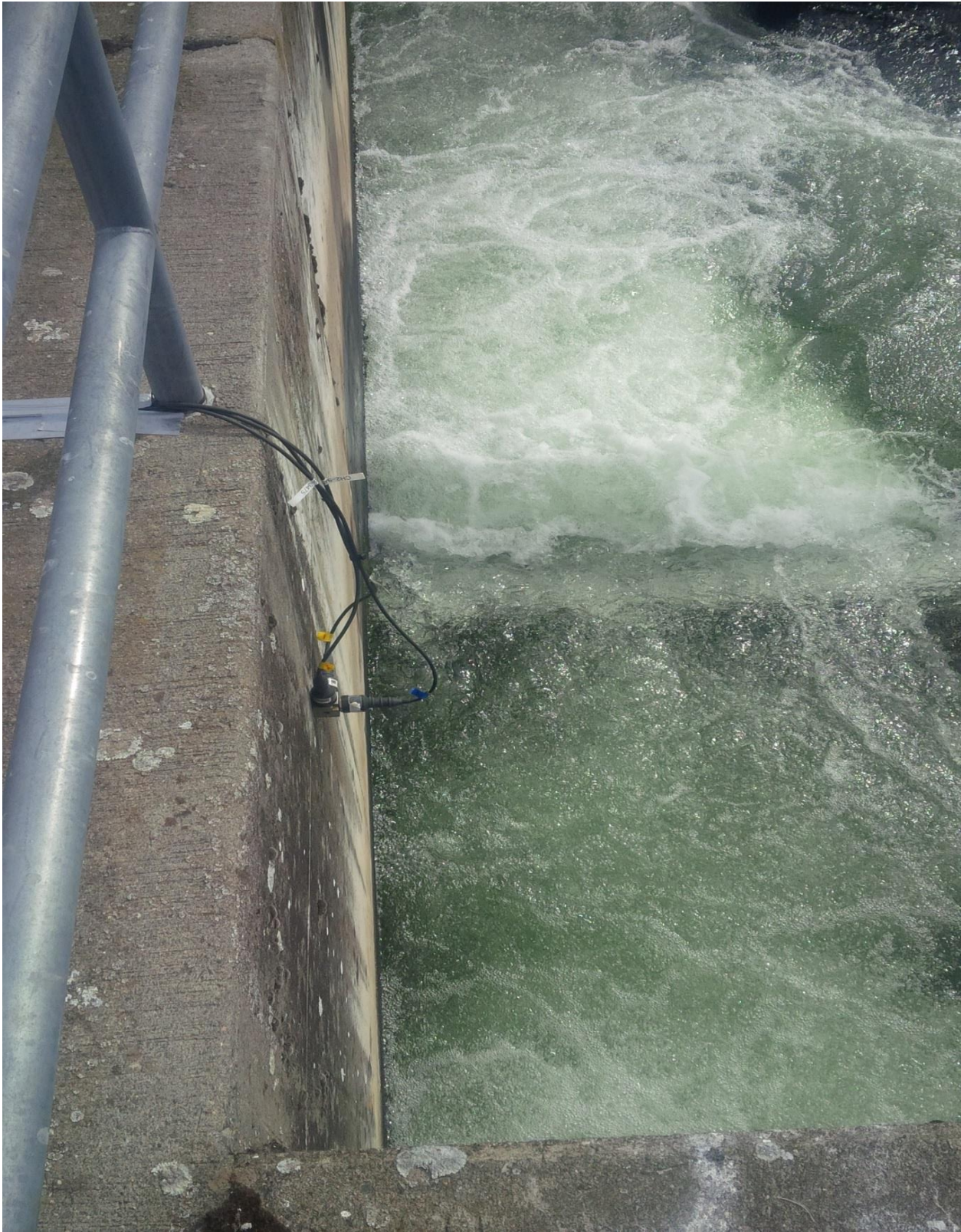
Vibration sensor on east fish ladder.
